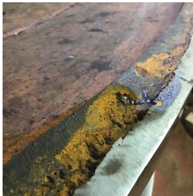
Figure 5-23: Runner Crown Cavitation Damage, VT-5
