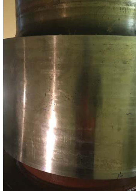
Figure 5-50: Turbine Shaft Bearing Journal, Light scratches
