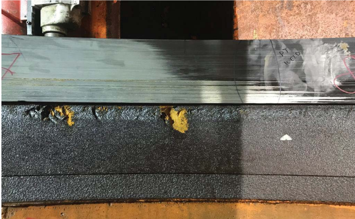
Figure 5-281: Bottom Ring Machined (Partial Clean)
