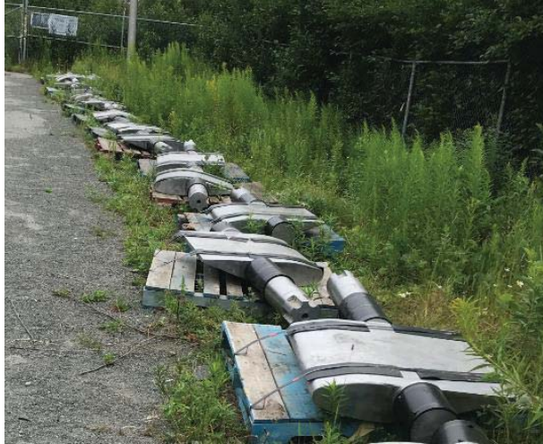
Figure 5-8: Finished Wicket Gates outside BDES Powerhouse 2
