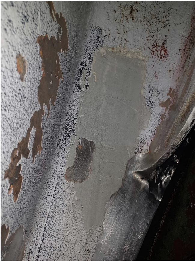
Photo 5: Cavitation Repairs on Runner Band using Belzona
