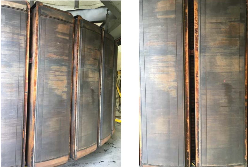
Figure 5-112: Rotor Pole: Rust and Oxidation
