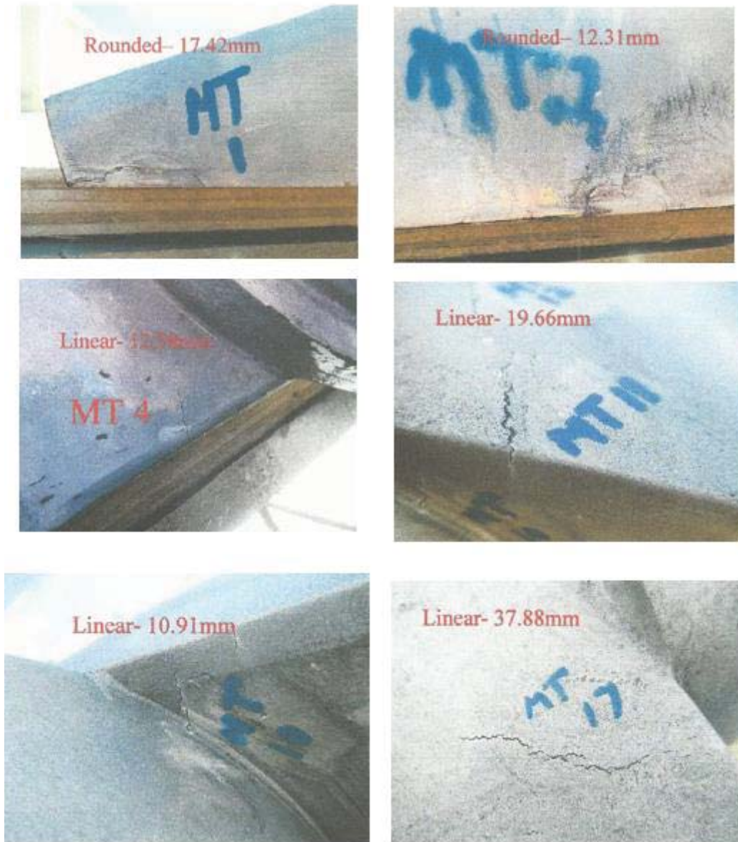
Figure 5-7: Wicket Gate #18 - MT Indications
