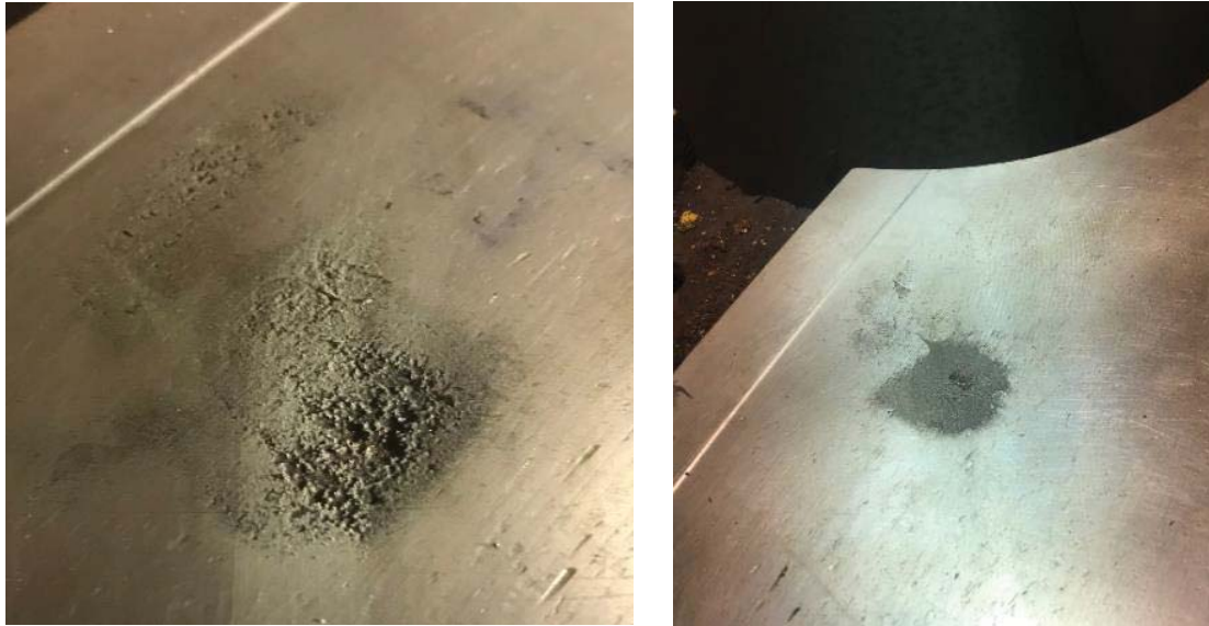
Figure 5-239: Bottom Ring, Water Passage Surface Cavitation
