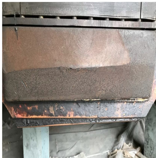
Figure 3-7: Dislodged Field Coil on Pole #20 (Source: 2019 Outage Report)
