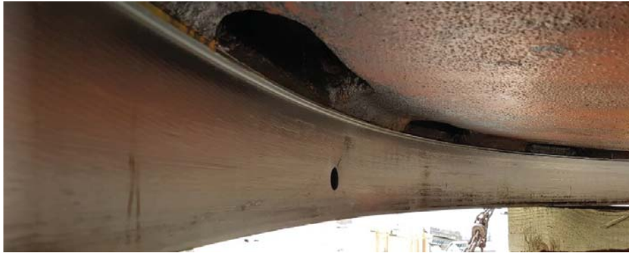
Figure 5-213: Head Cover, Wearing Ring Scratches and Scoring
