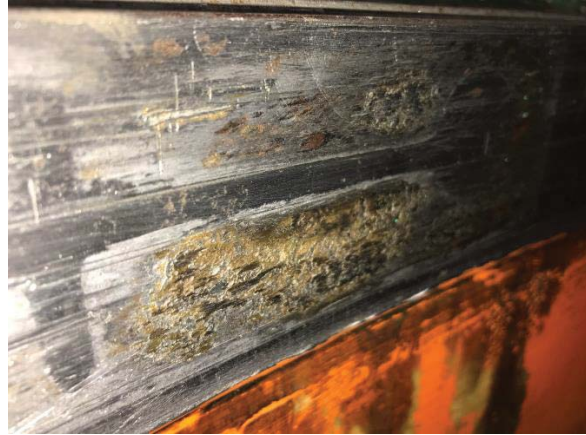
Figure 5-63: Operating Ring, Upper Bearing Surface Damage
