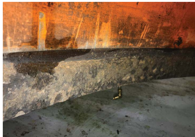
Figure 5-64: Operating Ring, Lower Bearing Surface Damage
