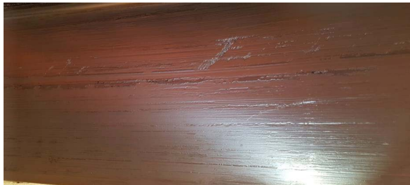
Figure 5-214: Head Cover, Wearing Ring Scratches and Scoring
