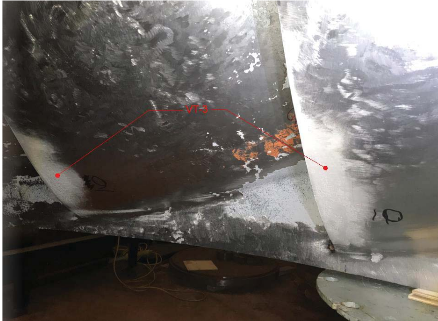
Figure 5-20: Runner Cavitation Damage, VT-3
