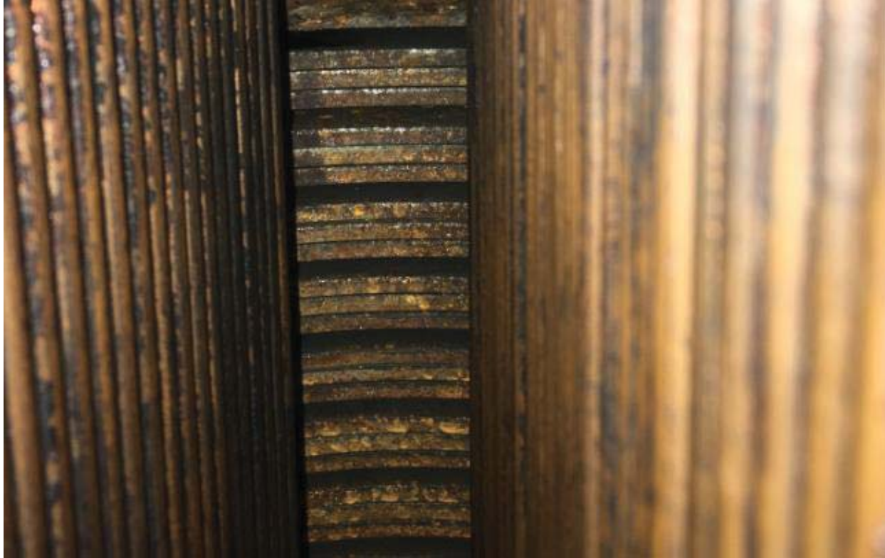
Figure 5-97: Rotor Rim, Outer condition of Rim Laminations (August 2019, Preassembly Oxidation)
