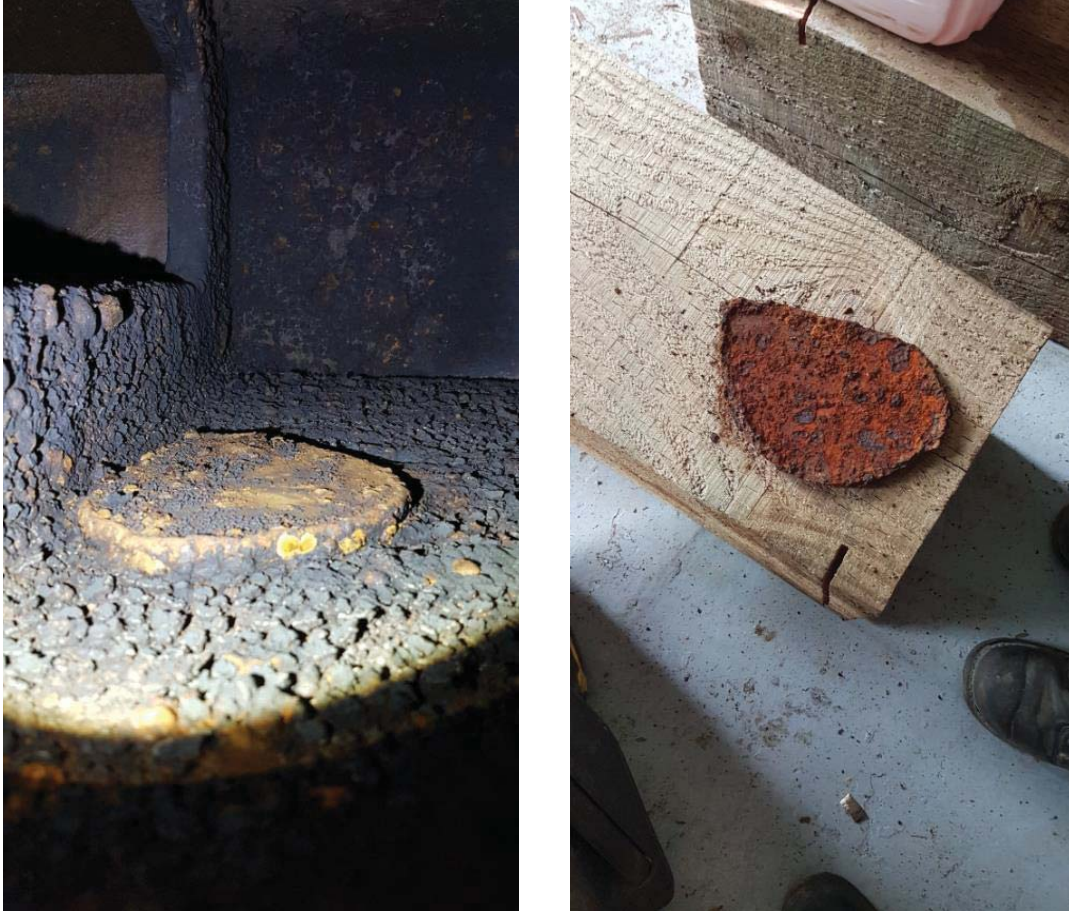
Figure 5-216: Head Cover, Runner Cover Balance Plate Steel Plate Found
