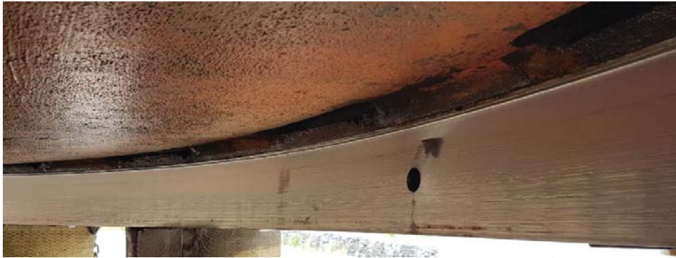
Figure 5-212: Head Cover, Wearing Ring Scratches and Scoring
