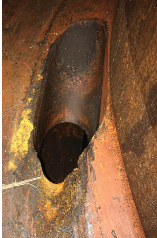
Figure 5-30: Runner Crown Pressure Relief Holes Cavitation Damage, VT-7
