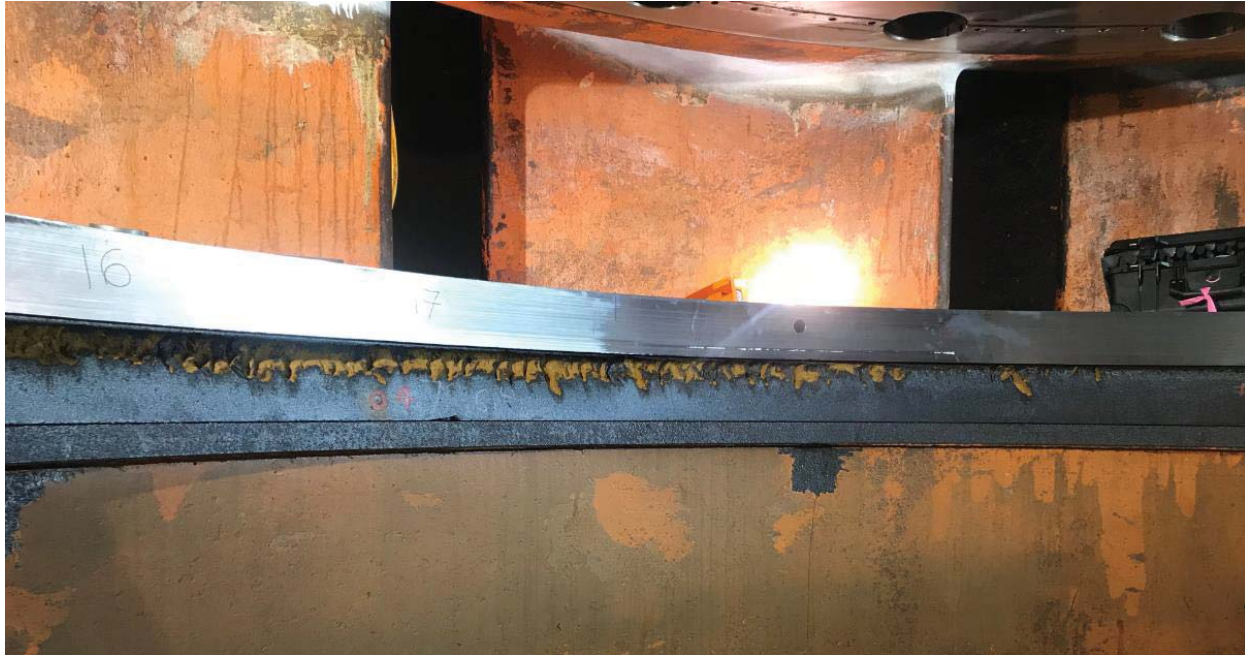
Figure 5-245: Bottom Ring, Cavitation Damage
