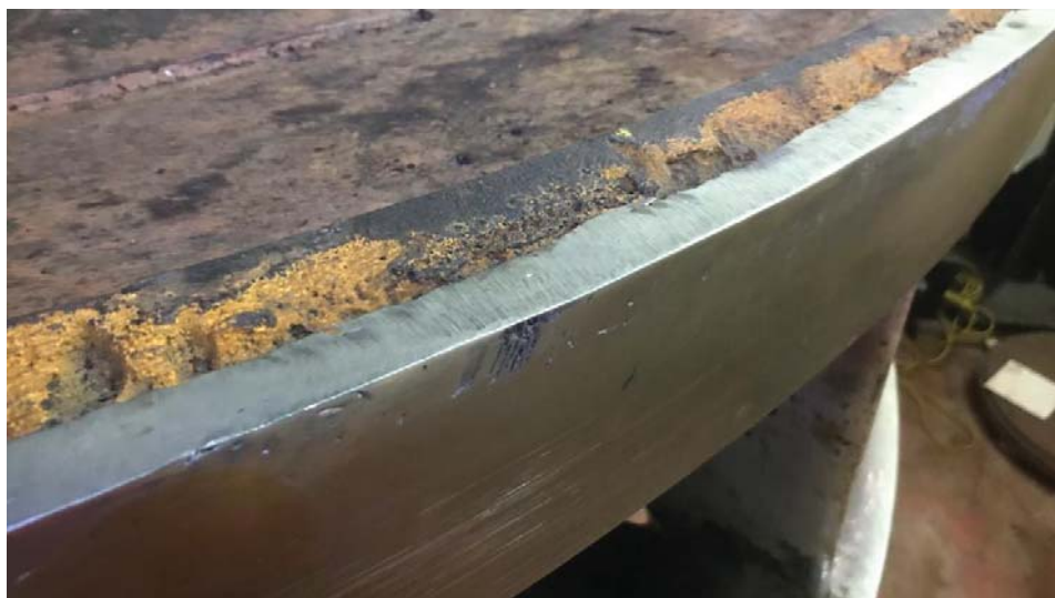
Figure 5-25: Runner Crown Cavitation Damage, VT-5
