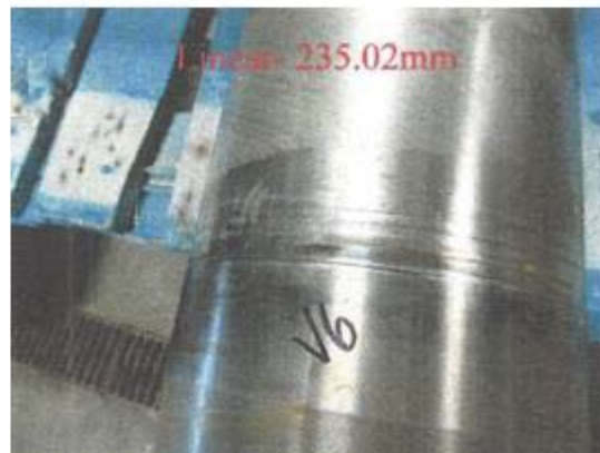
Figure 5-2: Visual Inspection - Typical Trunnion Indications
