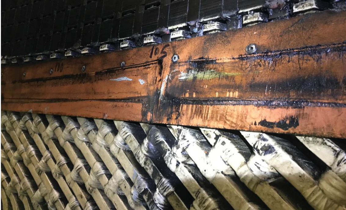
Figure 5-141: Stator Windings: Typical Grease and Oil on Bottom End of Windings
