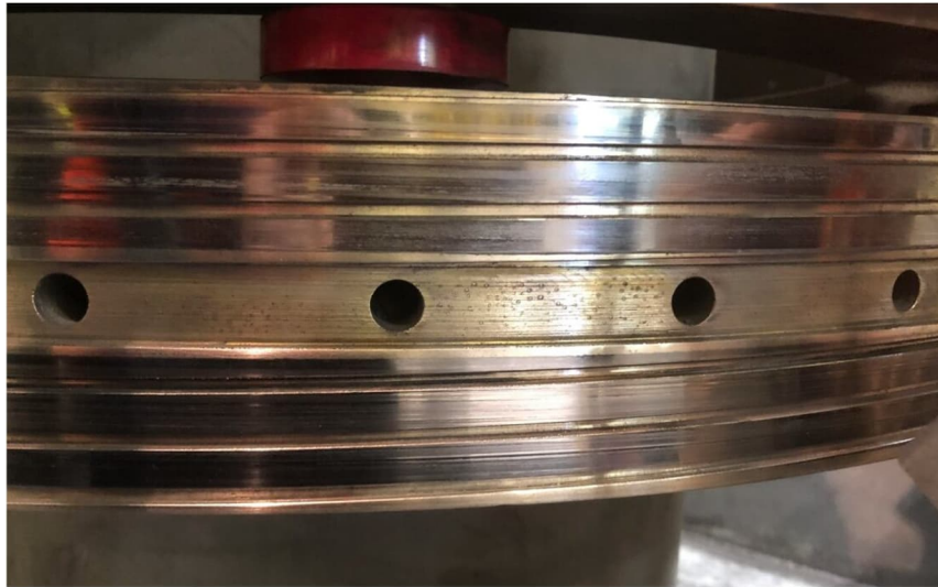
Figure 3-44: Typical condition of the Slip Rings (no concerns to note)
