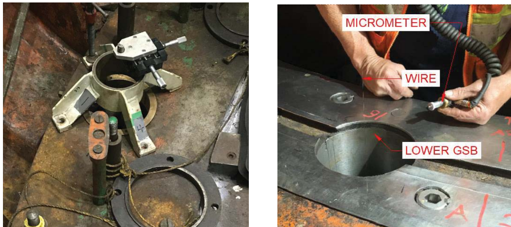
Figure 5-261: Wire Micrometer Example
