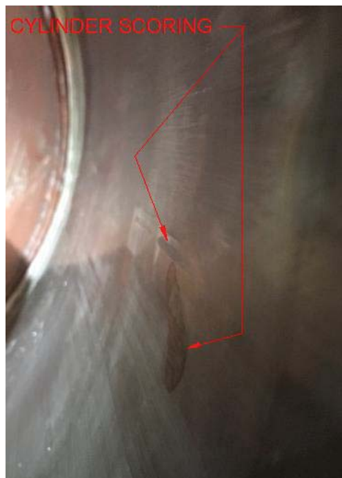
Figure 5-76: Servomotor, Cylinder Scoring
