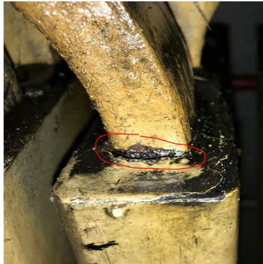
Figure 3-4: Example of Cracks at the Edges of End-Winding Caps
