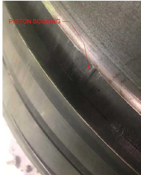
Figure 5-75: Servomotor, Piston Scoring
