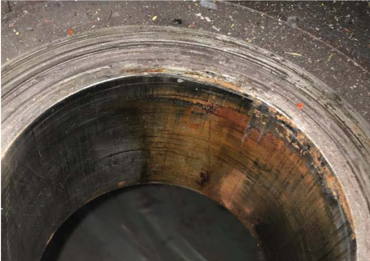
Figure 5-88: Rotor Hub, Coupling Hole Fretting
