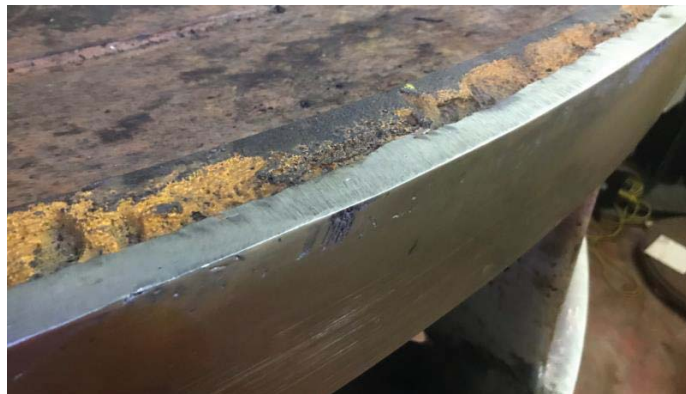
Figure 5-22: Runner Crown Cavitation Damage, VT-5
