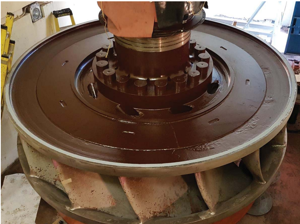
Figure 5-44: Runner Balance Cover Plate Repaired
