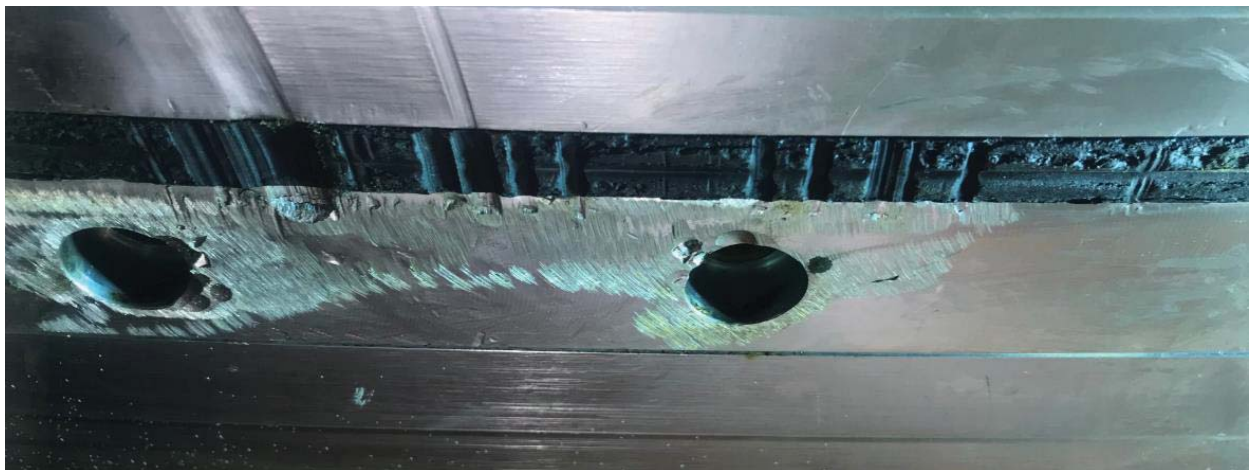
Figure 5-218: Head Cover, Wicket Gate Seals and Seal Retaining Plates (Damage)
