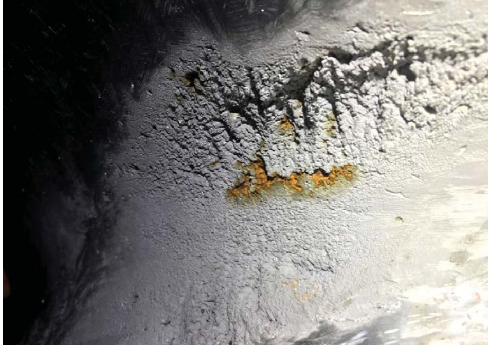
Figure 5-18: Runner Bucket Cavitation, VT-2
