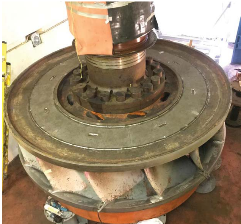
Figure 5-43: Runner Balance Cover Plate Welded
