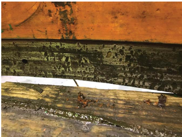
Figure 5-64: Operating Ring, Lower Bearing Surface Damage
