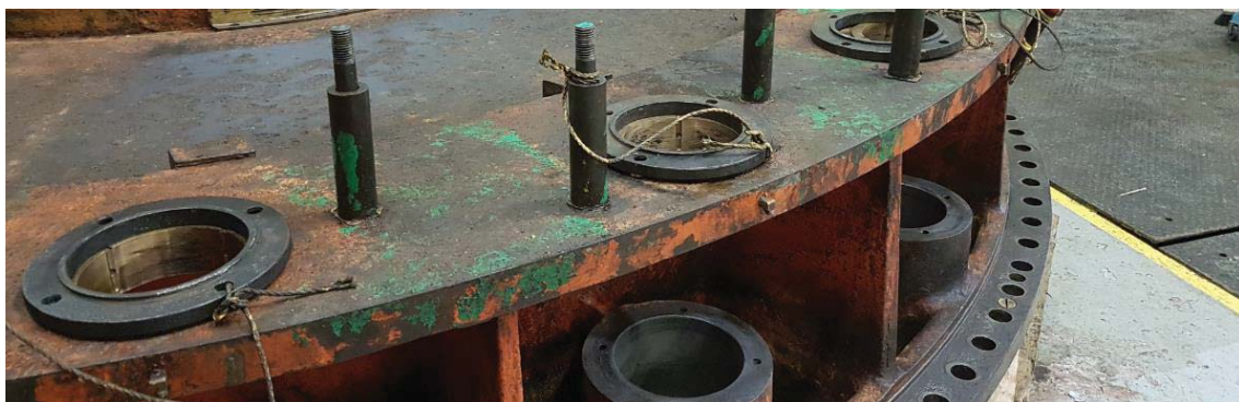
Figure 5-200: Head Cover, Paint Condition of Bolting Flange
