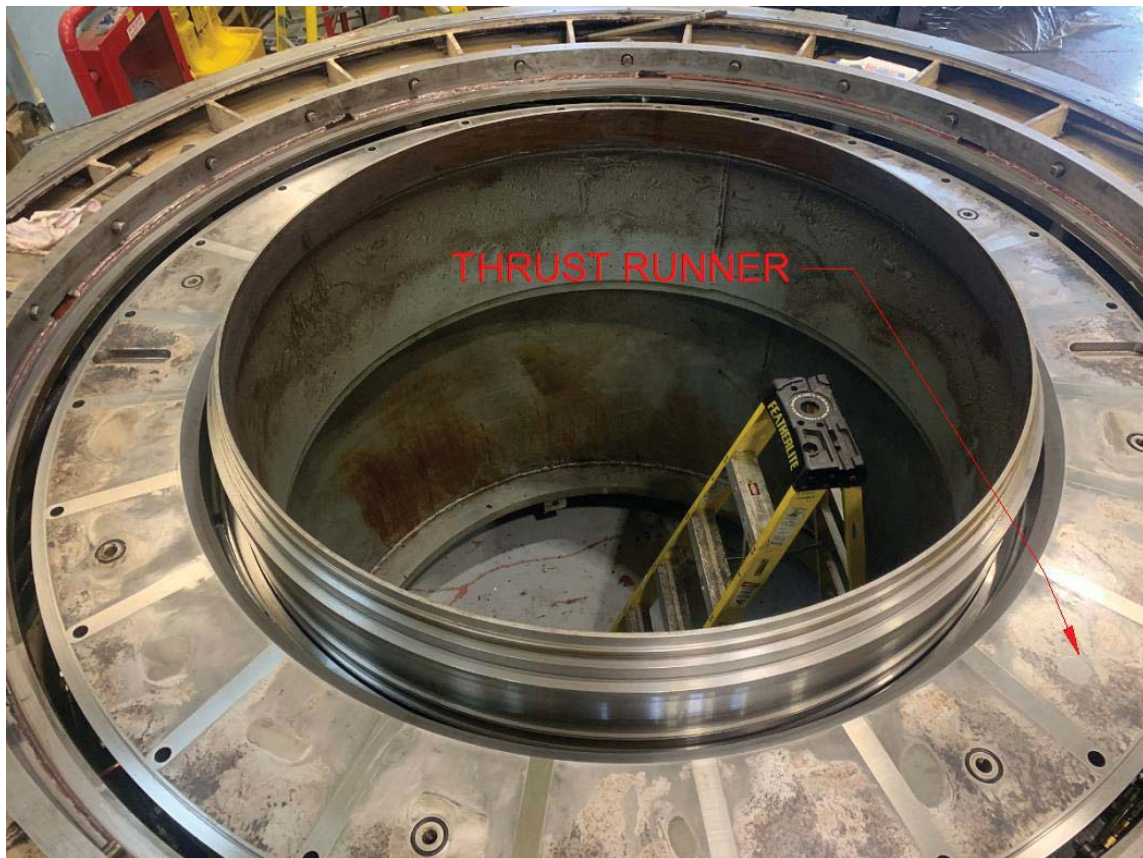
Figure 5-186: Thrust Runner, after reassembly into Unit.
