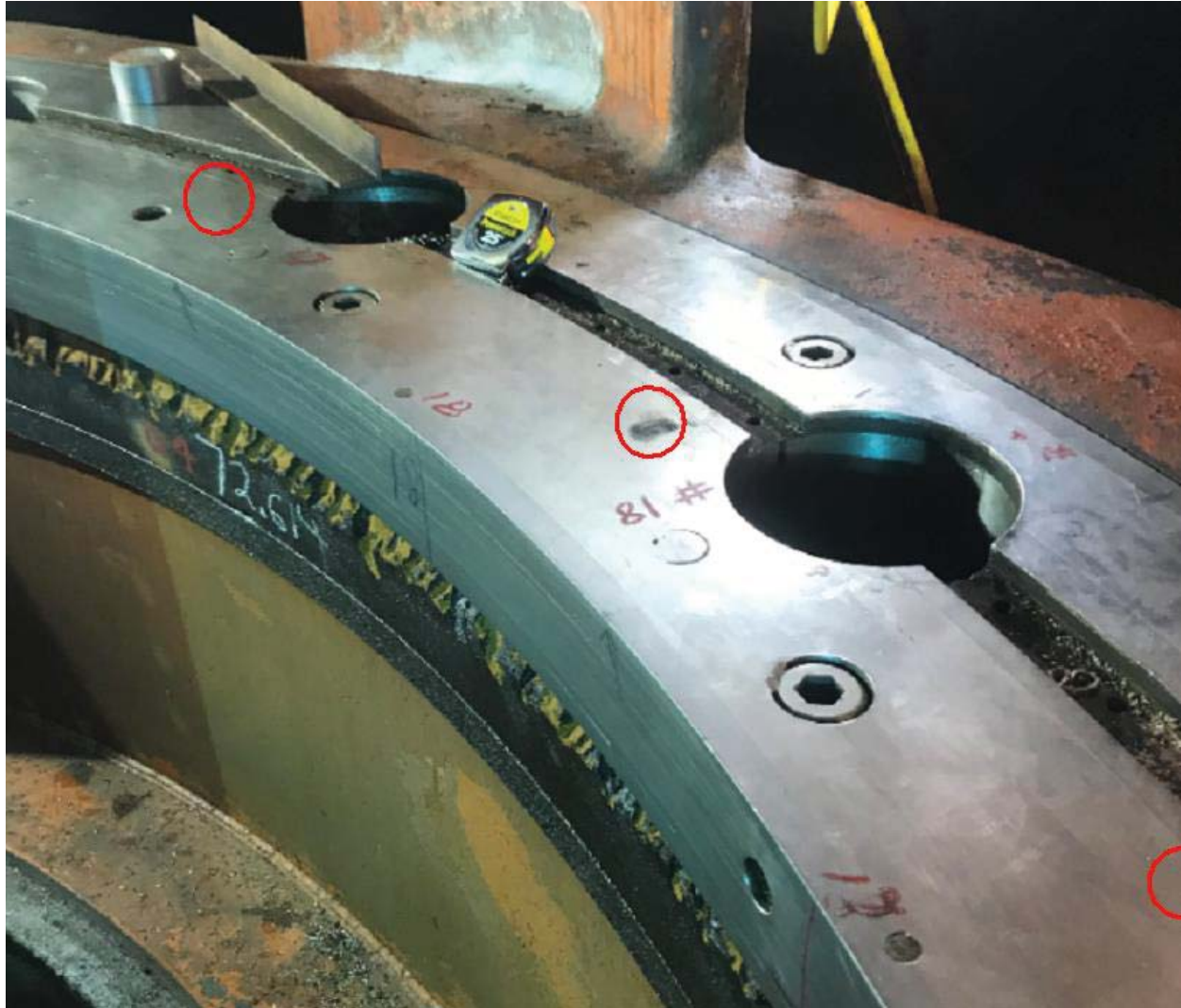
Figure 5-238: Bottom Ring, Water Passage Surface Cavitation
