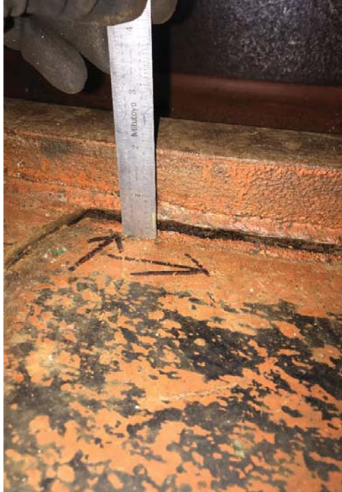
Figure 5-28: Balance Plate Cracks, VT-6
