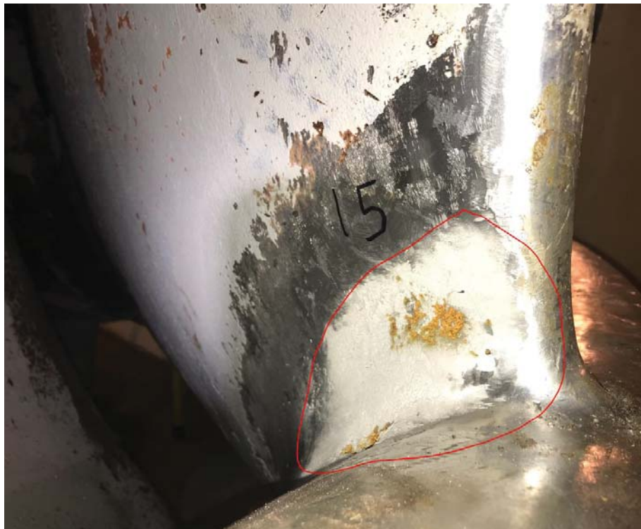
Figure 5-19: Runner Cavitation Damage, VT-2
