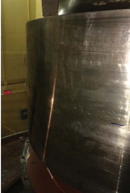
Figure 5-50: Turbine Shaft Bearing Journal, Light scratches
