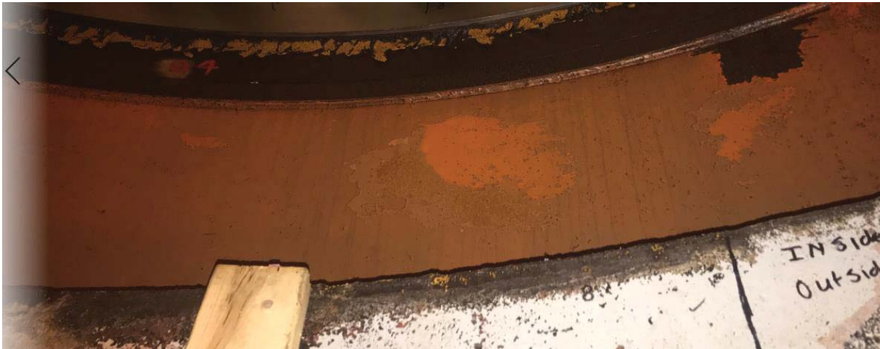
Figure 5-290: Discharge Ring, Rust and Corrosion
