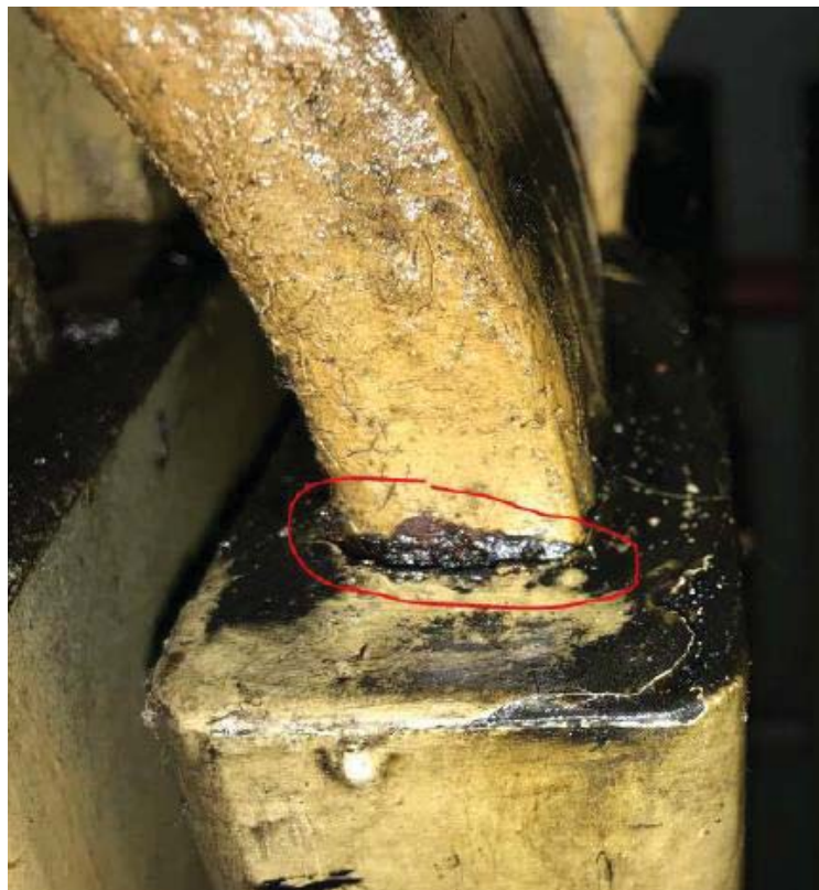
Figure 5-144: Stator Windings: End-Cap Insulation Cracked
