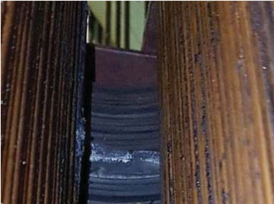
Figure 5-108: Rotor Pole: Melting Rim Laminations
