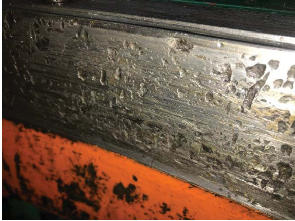
Figure 5-63: Operating Ring, Upper Bearing Surface Damage
