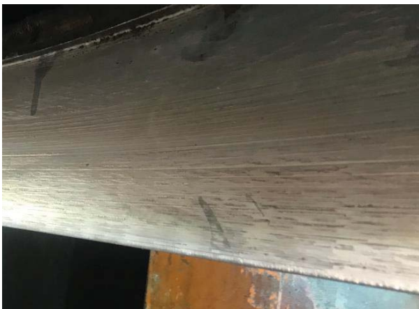
Figure 5-272: Head Cover Wearing Ring Condition (Upper)
