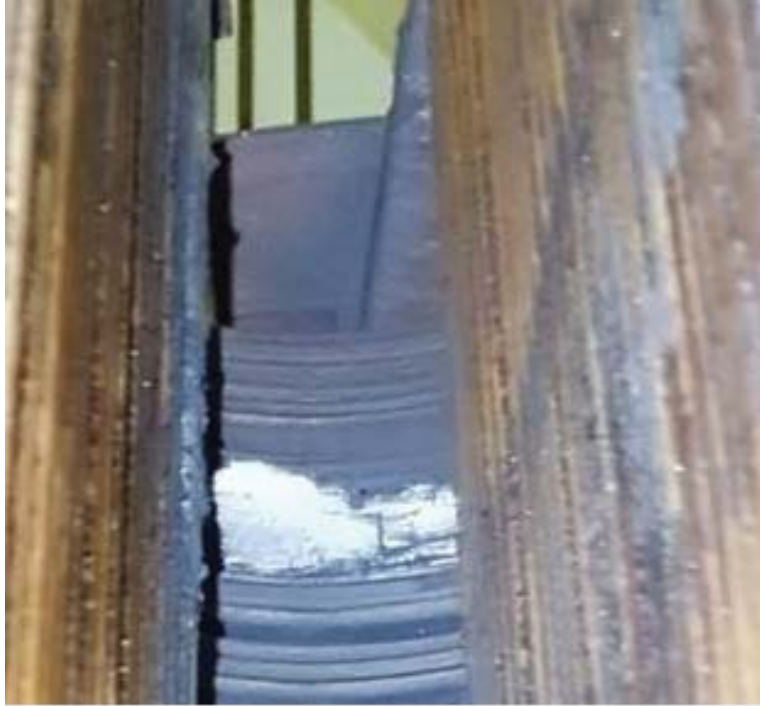
Figure 5-109: Rotor Pole: Melting Rim Laminations
