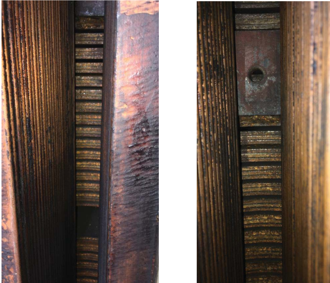
Figure 5-114: Rotor Poles: Rim Rust and Oxidation
