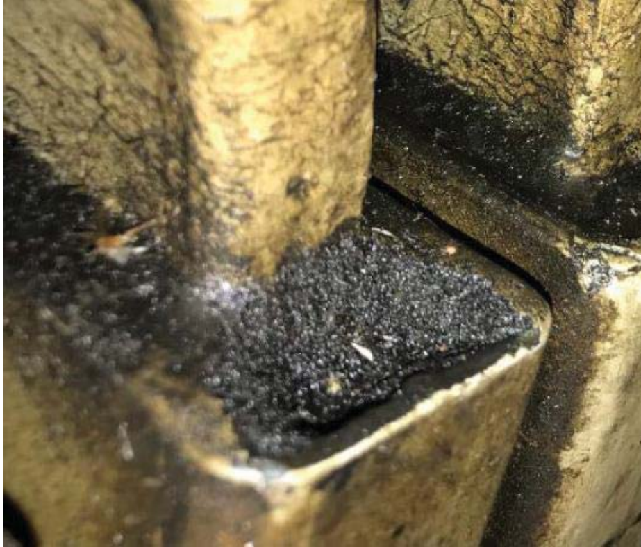
Figure 5-145: Stator Windings: Damaged End-Cap
