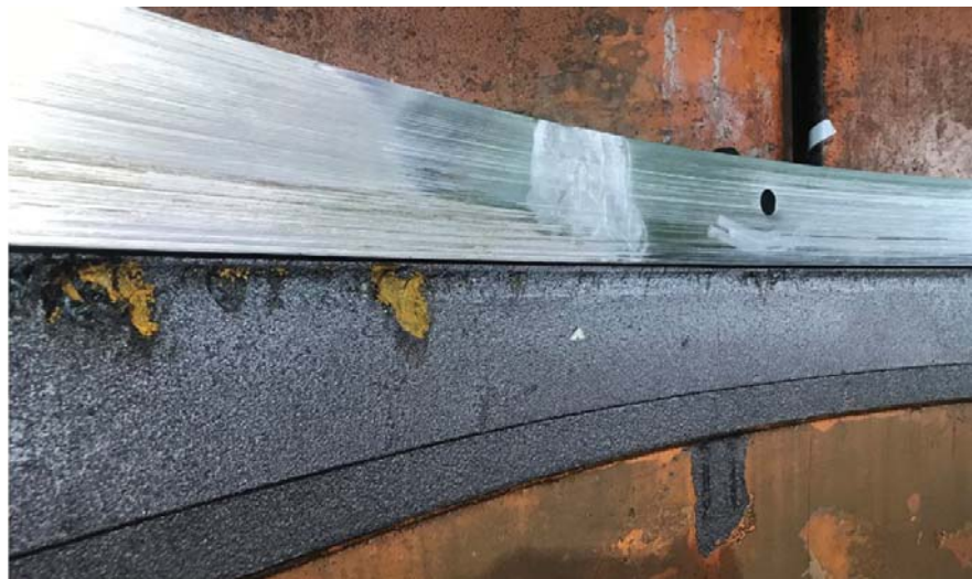
Figure 5-280: Bottom Ring Machined (Partial Clean)
