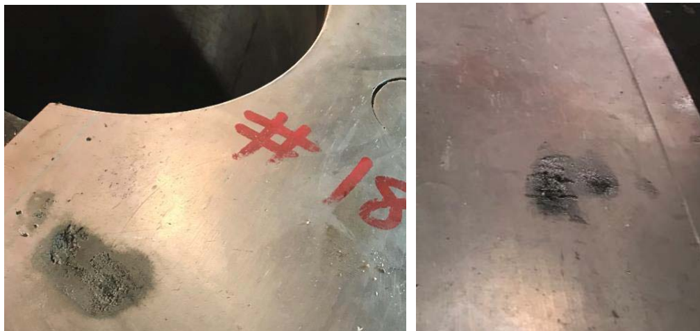
Figure 5-240: Bottom Ring, Water Passage Surface Cavitation
