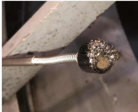
Figure 3-5: Example of Magnetic Metallic Debris Deposited on Top of the Bottom End-Winding Caps, Collected with a Magnet
