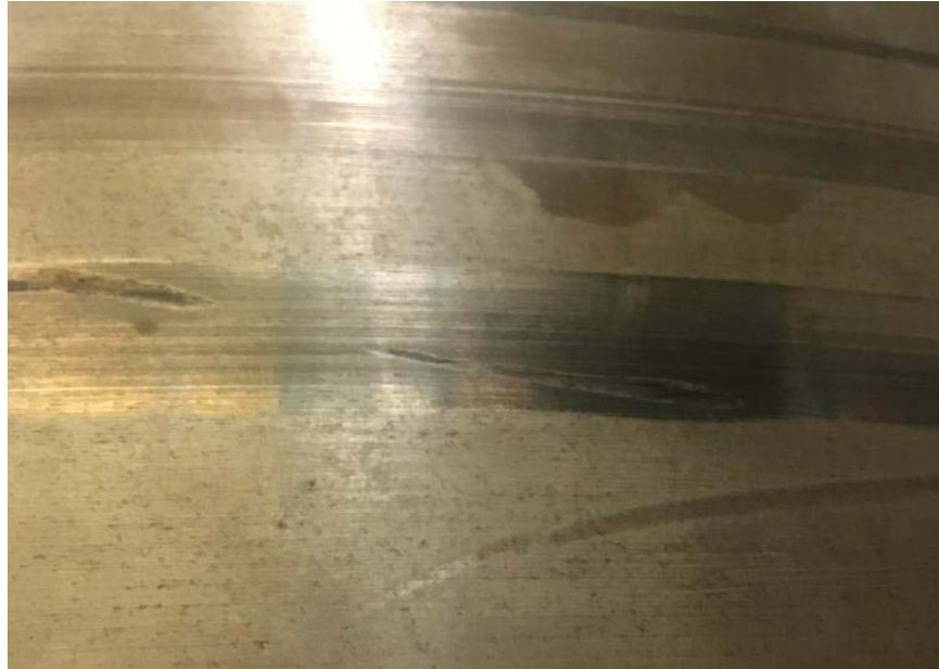
Figure 5-54: Generator Shaft, Light Scratches
