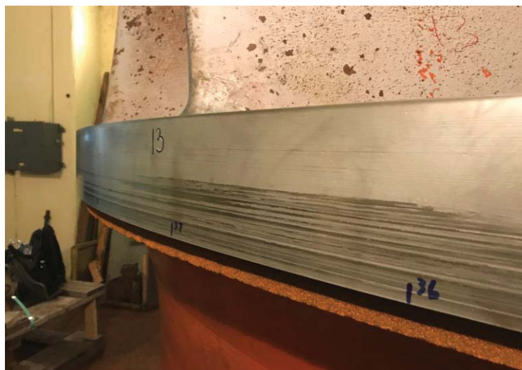
Figure 5-34: Runner Lower Wearing Ring, Contact Damage
