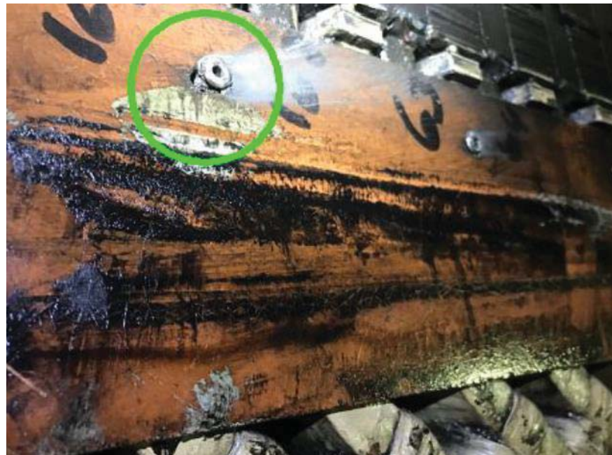
Figure 5-134: Stator Core, Loose Rivet beginning to pull through Air Guide
