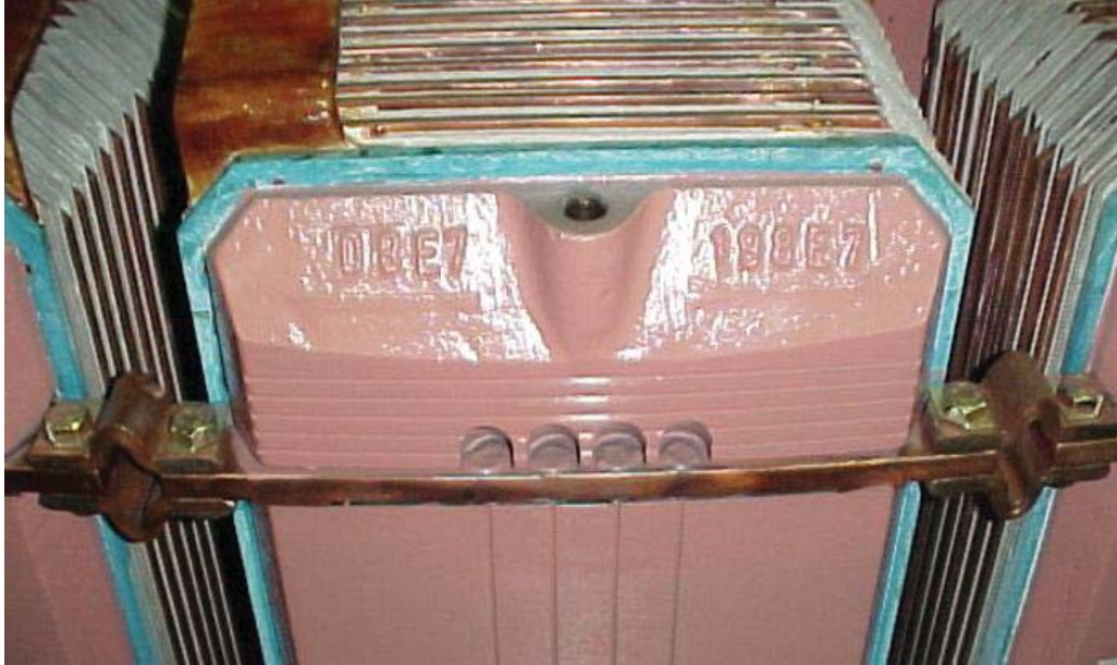
Figure 5-103: Rotor Pole Example: Voith picture of a new poles.
