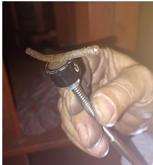
Figure 3-1: Example of Typical Magnetic Debris (Piece of Welding Rod) Found on the Shelves of the Stator Frame
