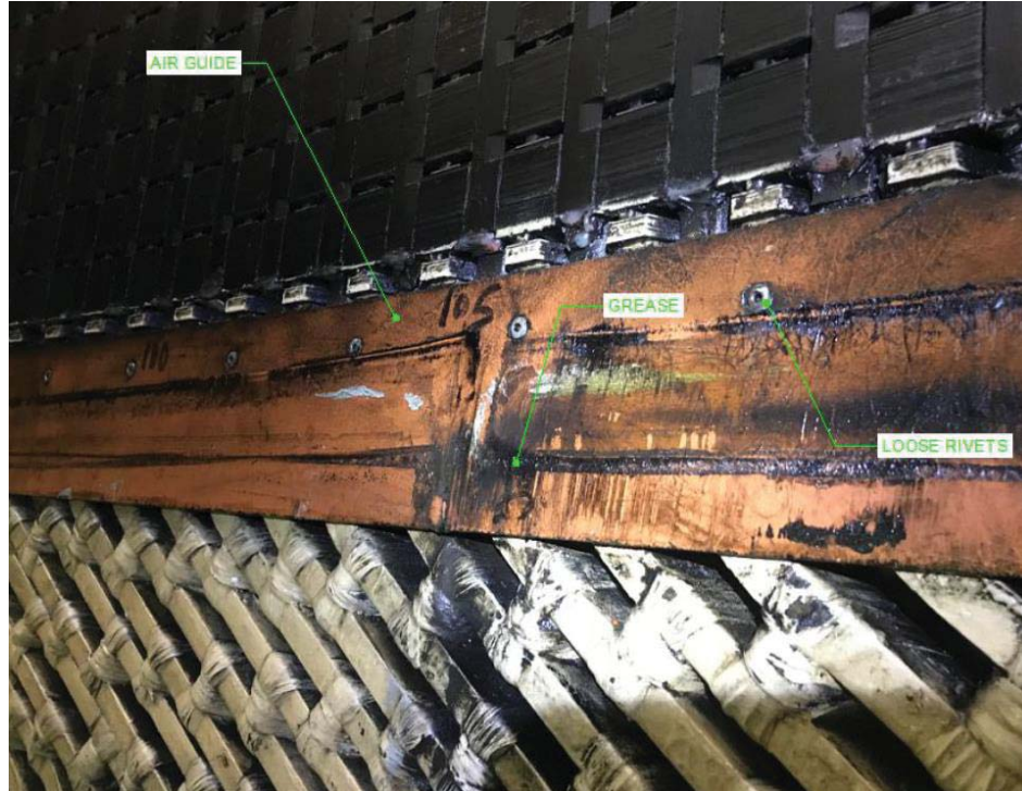
Figure 5-133: Stator Core, Air Guide
