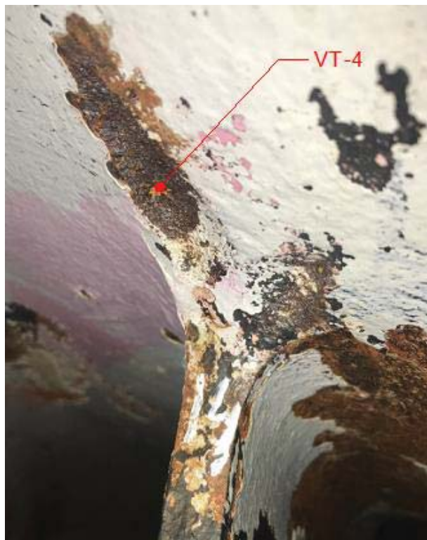
Figure 5-21: Runner Bucket Cavitation Damage, Discharge Edge near Crown, VT-4
