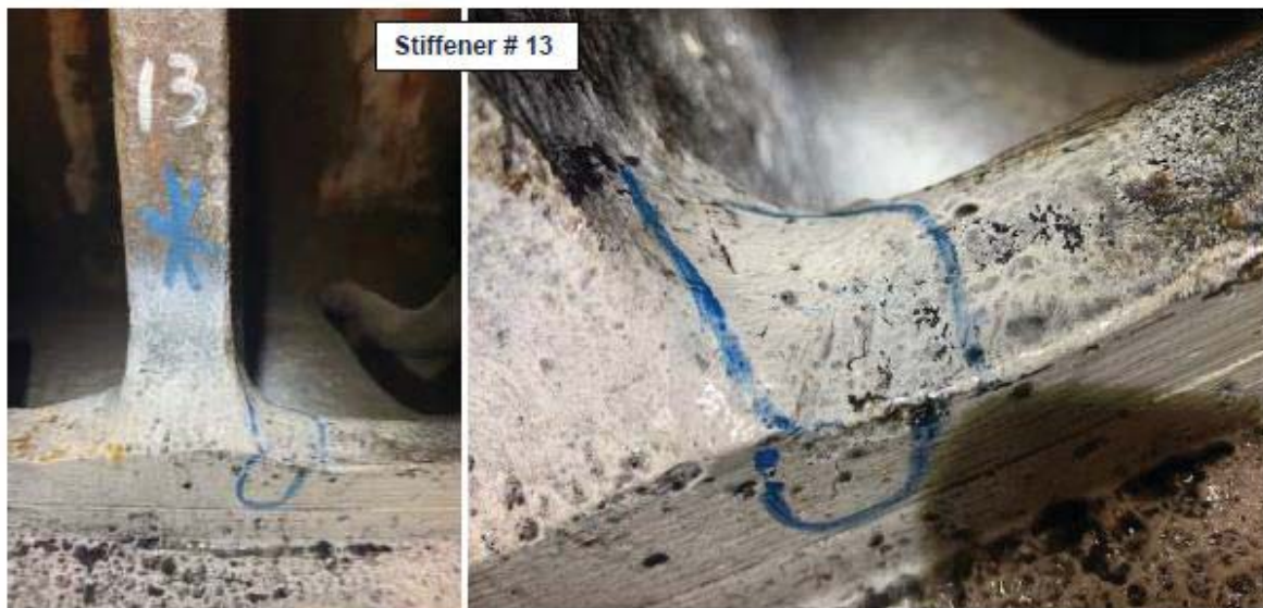
Figure 5-230: Head Cover, Small Stiffener Cracks
