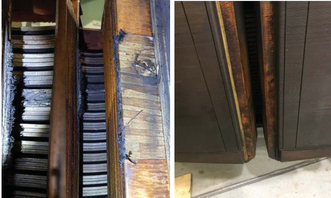
Figure 5-101: Rotor Pole, (Left) Damaged Tape, (Right) Film of Dirt and Grease
