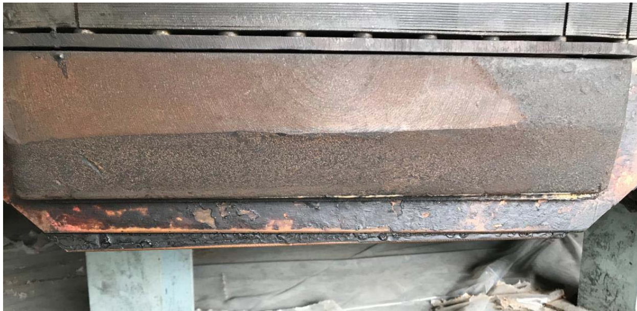
Figure 5-106: Rotor Pole: Dislodged Winding
