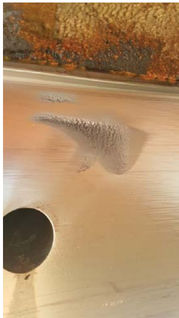
Figure 5-211: Head Cover, Wearing Ring Cavitation
