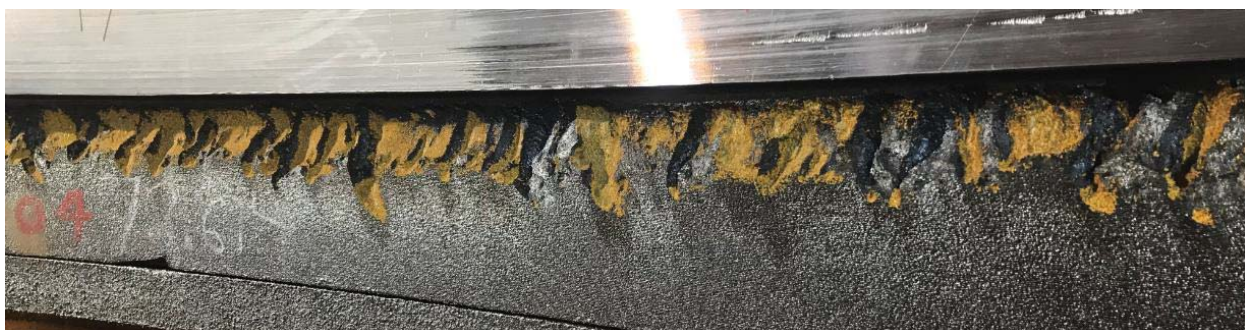
Figure 5-247: Bottom Ring, Cavitation Damage
