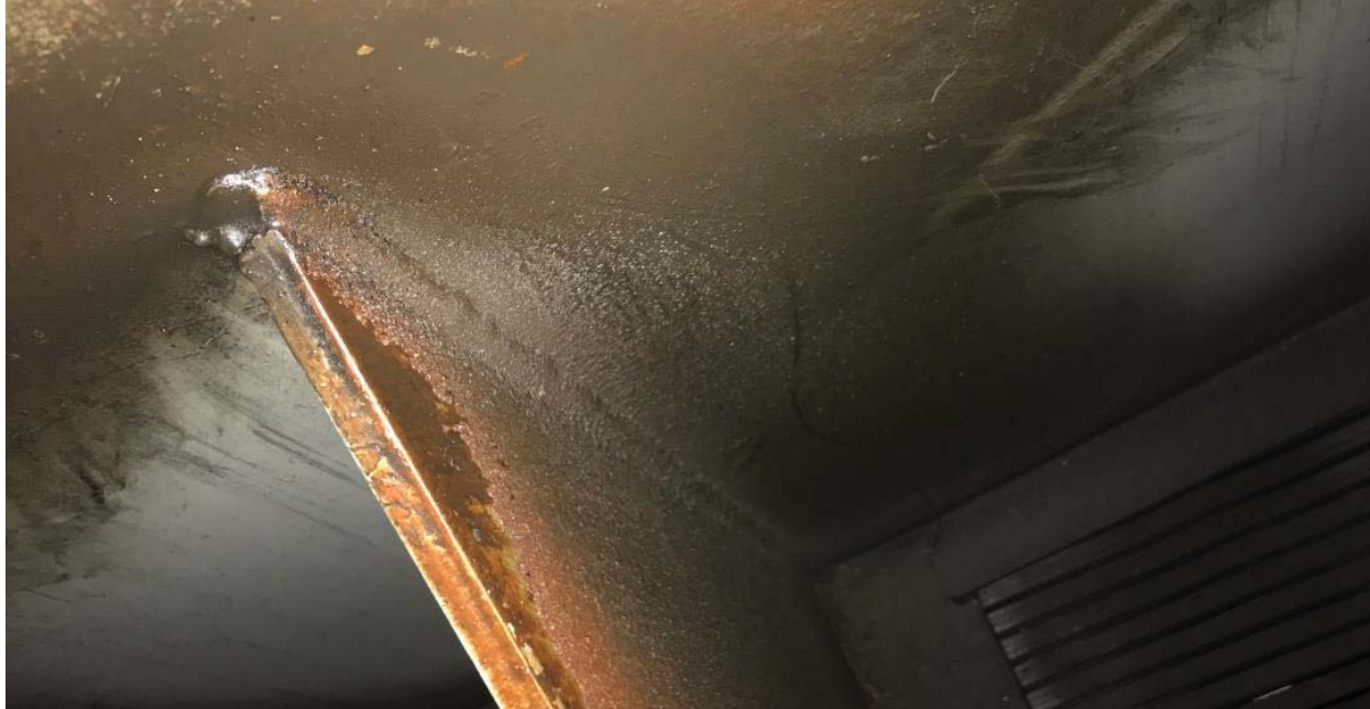
Figure 5-90: Rotor Hub, Oil Film, Grease, and Dirt
