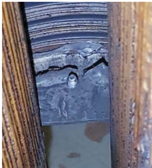
Figure 5-110: Rotor Pole: Melting Rim Laminations
