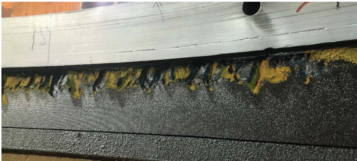
Figure 5-274: Bottom Ring Cavitation Damage
