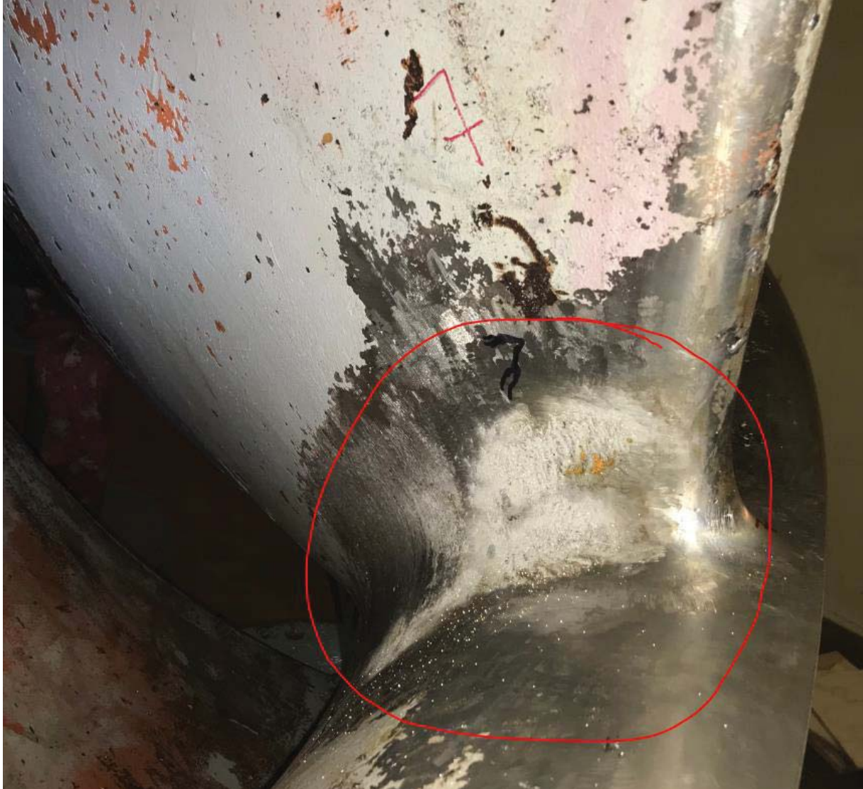
Figure 5-17: Runner Bucket Cavitation, VT-2
