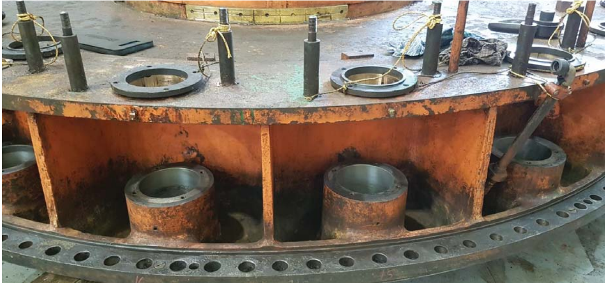
Figure 5-198: Head Cover, Paint Condition and Overall Appearance
