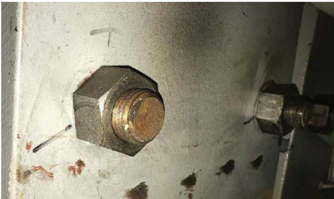
Figure 5-132: Stator Core, Pressure Plate Nut Movement
