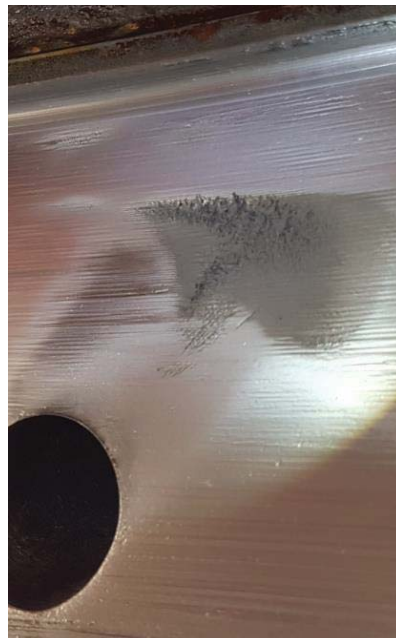
Figure 5-211: Head Cover, Wearing Ring Cavitation
