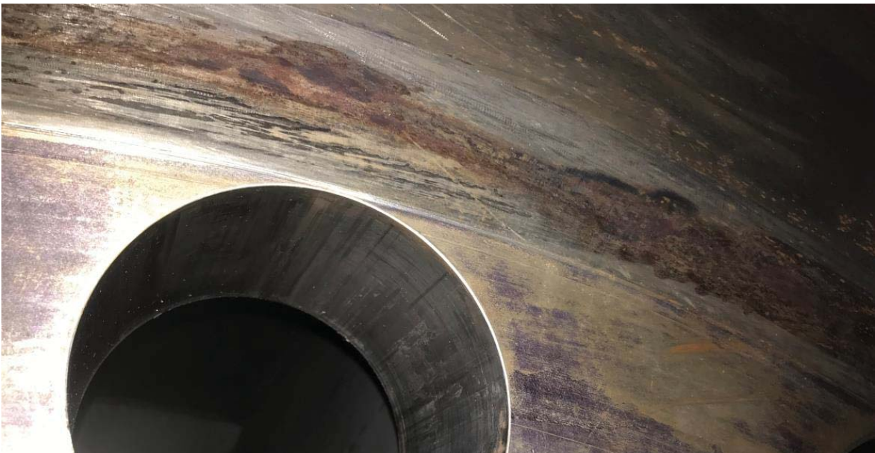
Figure 5-87: Rotor Hub, Light Fretting and Oxidation on Coupling Flange
