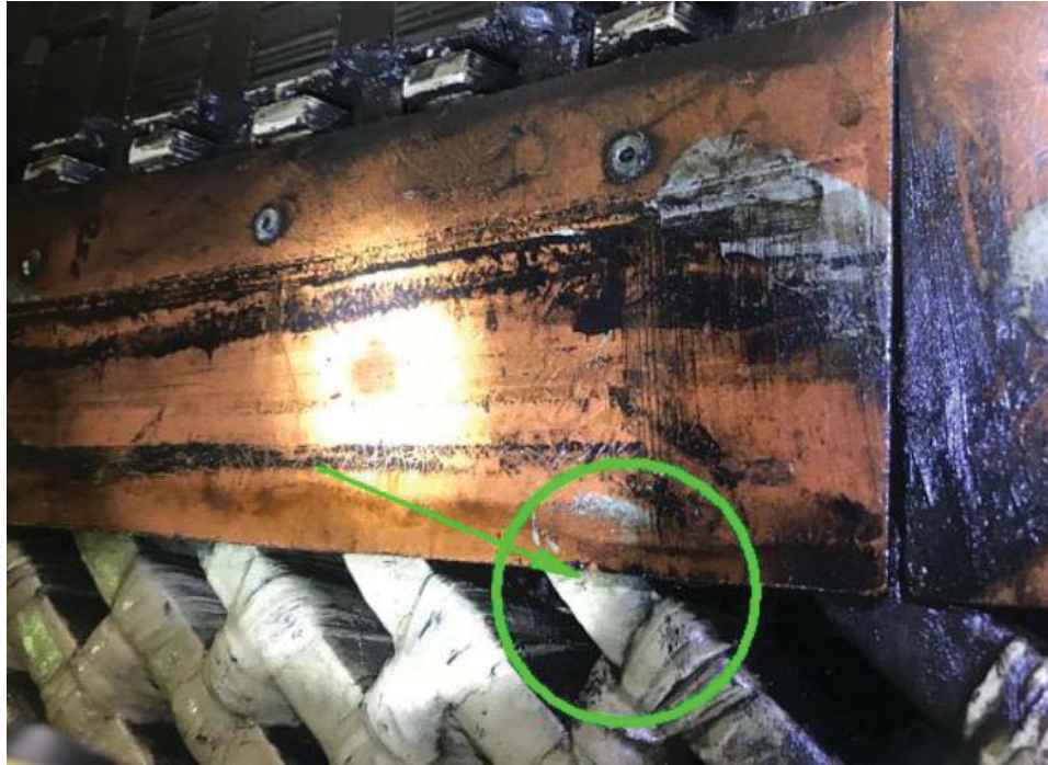
Figure 5-135: Stator Core, Air Guide Rubbing on Winding, due to Loose Hardware
