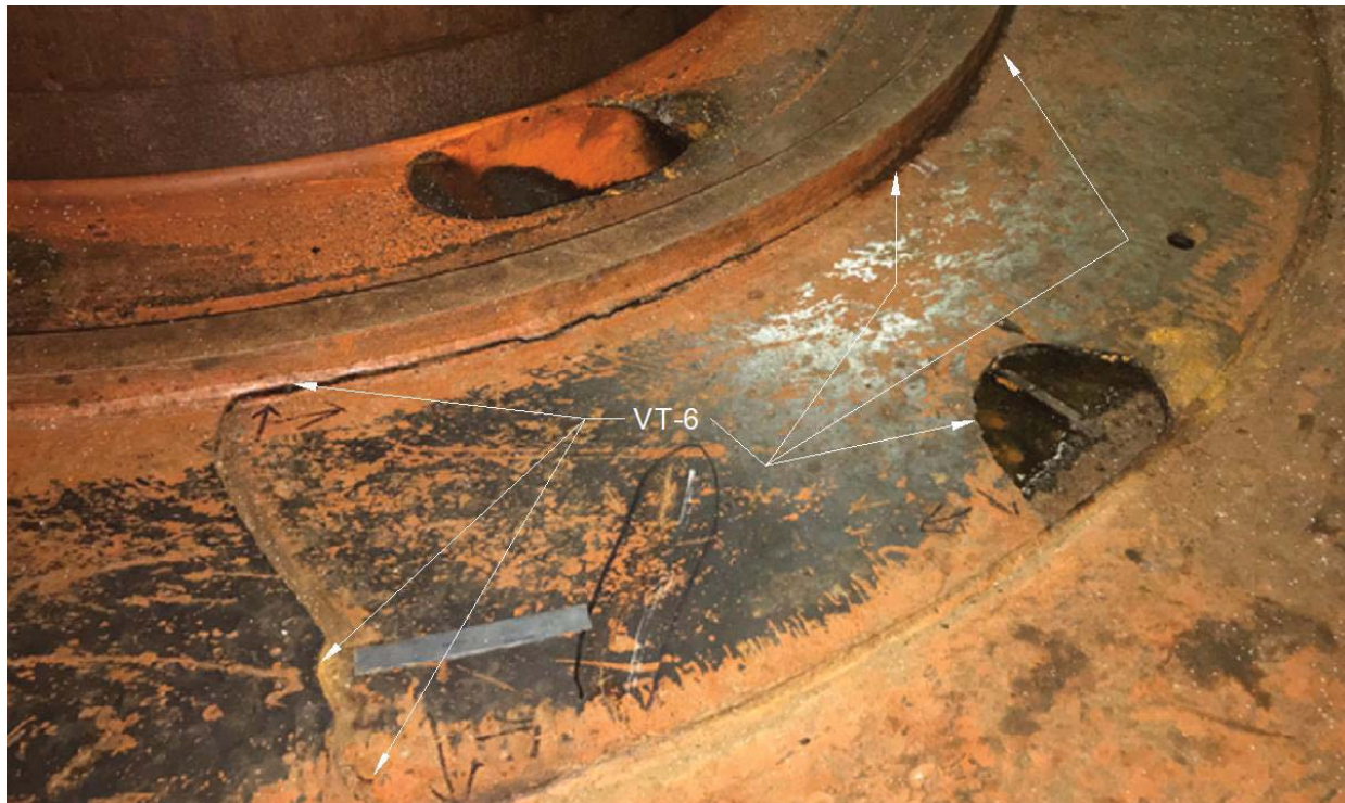
Figure 5-26: Runner Crown Balance Plate Damage, VT-6
