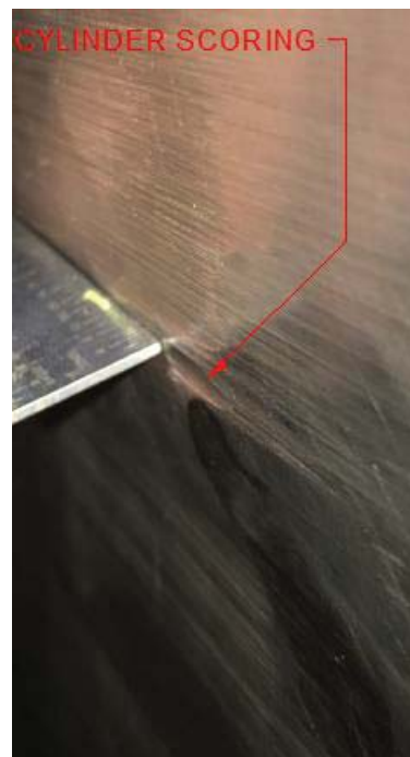
Figure 5-76: Servomotor, Cylinder Scoring
