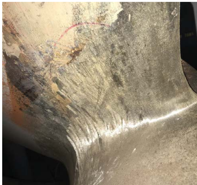
Figure 5-40: Runner Bucket Post Cavitation Repair
