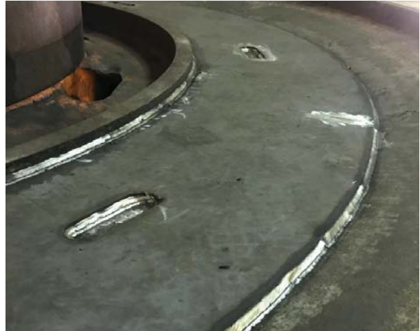
Figure 5-44: Runner Balance Cover Plate Repaired
