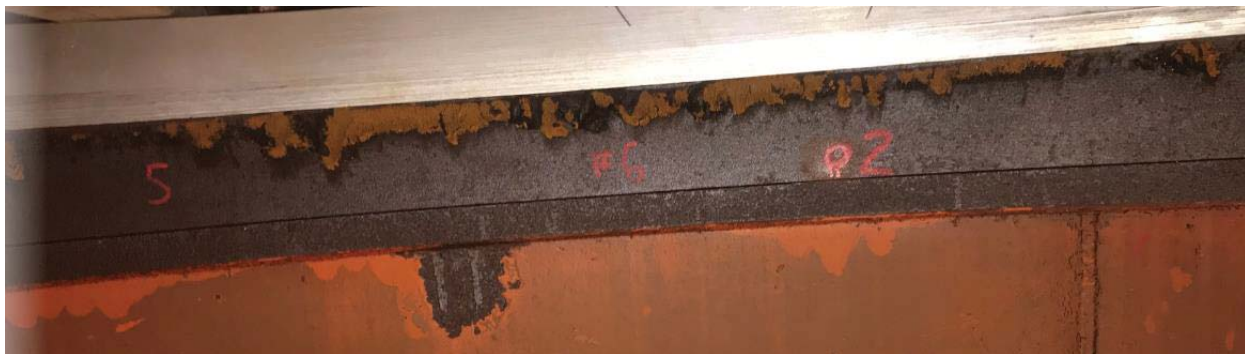
Figure 5-246: Bottom Ring, Cavitation Damage
