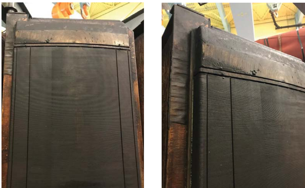
Figure 5-100: Rotor Pole, Film of Dirt and Grease
