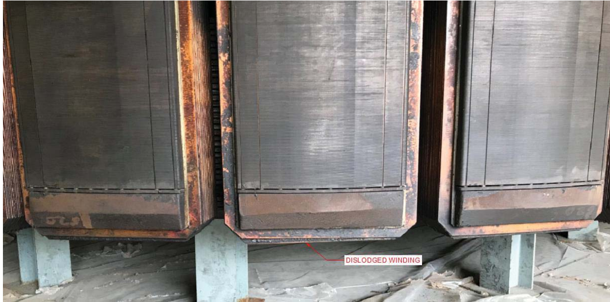
Figure 5-105: Rotor Pole: Dislodged Winding
