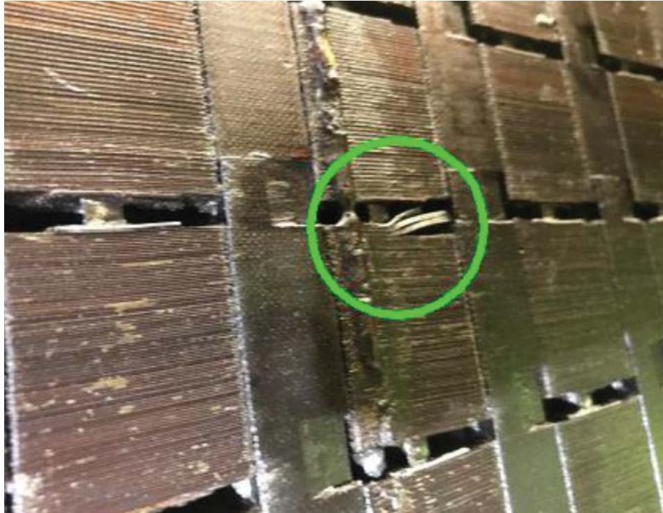
Figure 5-137: Stator Core, Bent Lamination Damage, the Cause was Unclear.
