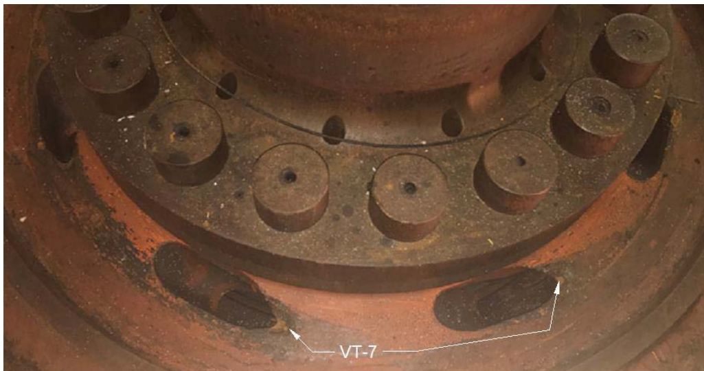
Figure 5-29: Runner Crown Pressure Relief Holes Cavitation Damage, VT-7
