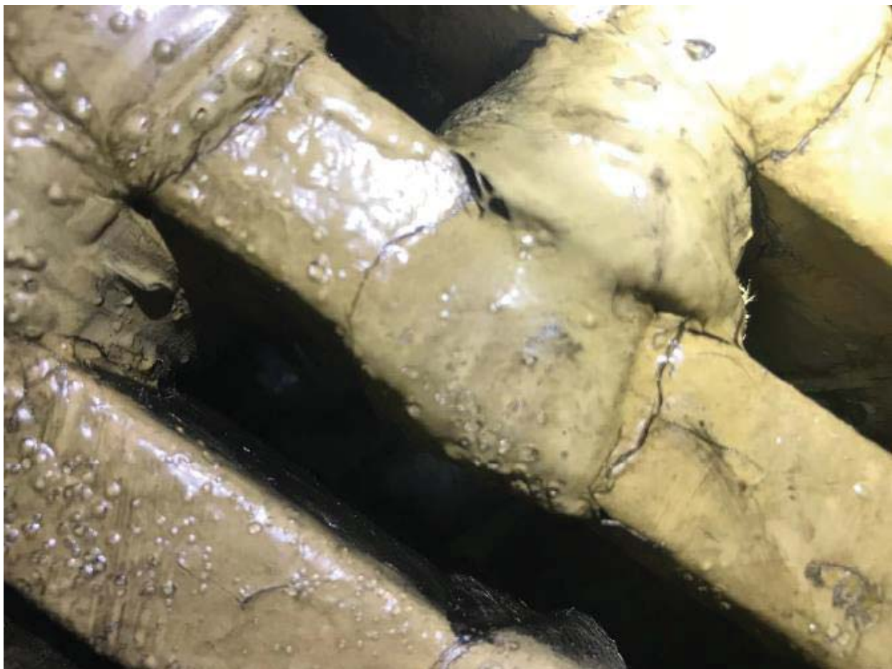
Figure 5-139: Stator Windings: Typical Insulation Cracking Found
