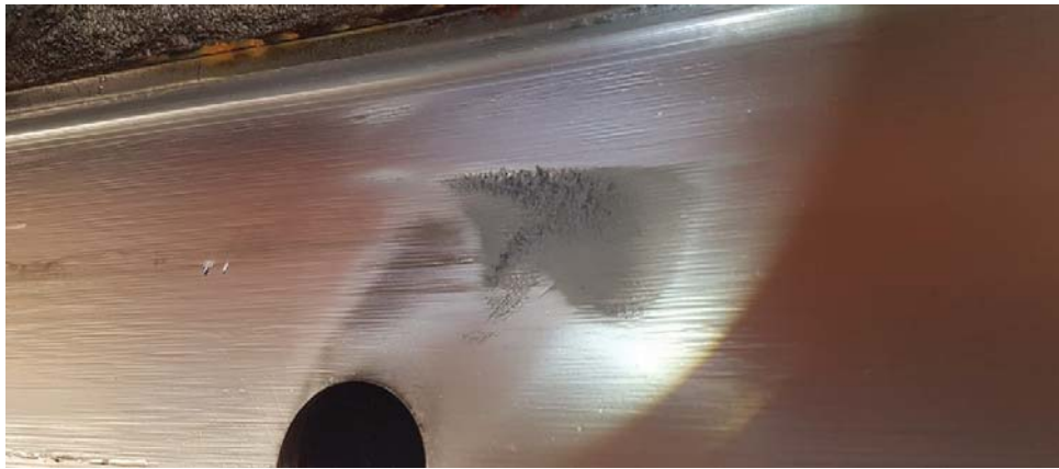
Figure 5-210: Head Cover, Wearing Ring Cavitation
