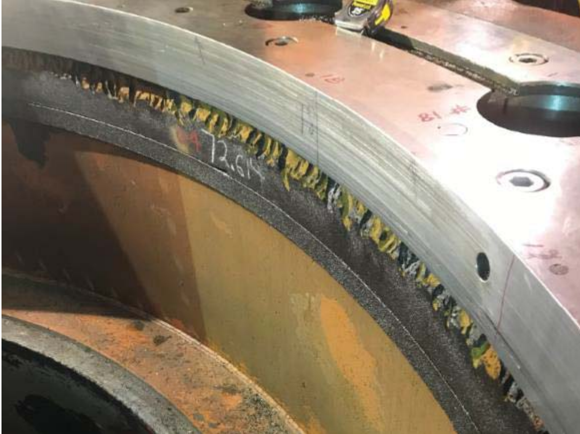
Figure 5-244: Bottom Ring, Wearing Ring Damage
