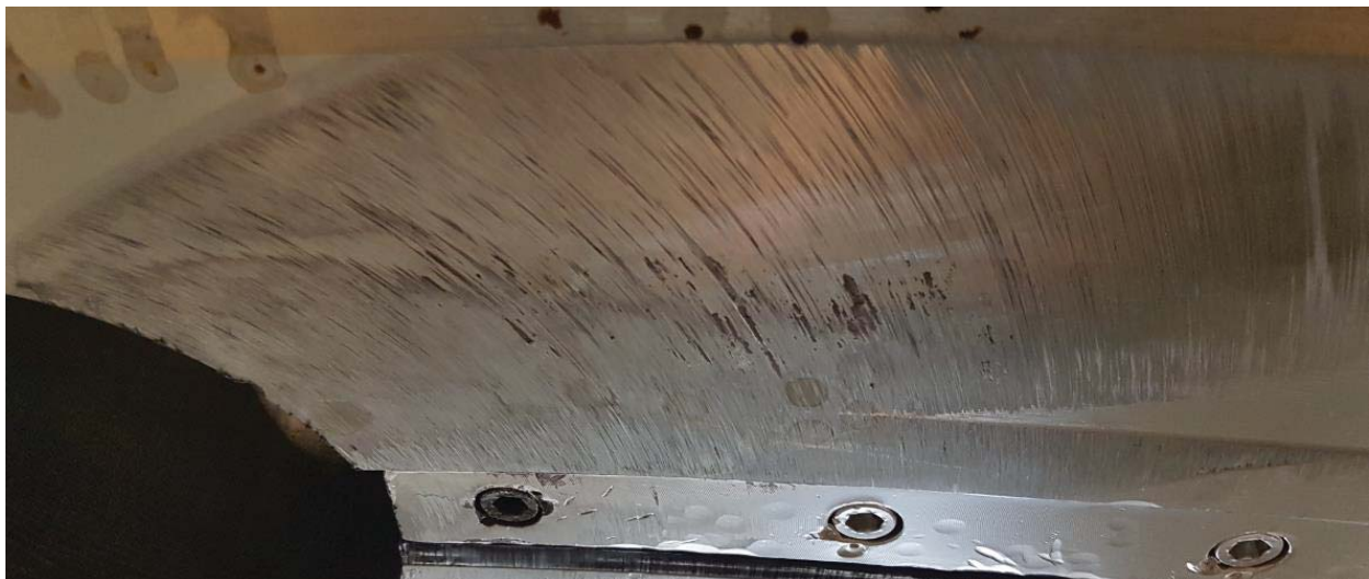
Figure 5-220: Head Cover, Water Passage Surface Damage
