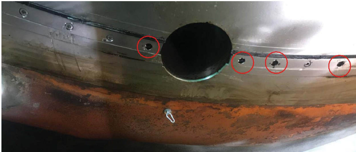
Figure 5-219: Head Cover, Seal Retaining Plates (Missing Screws)
