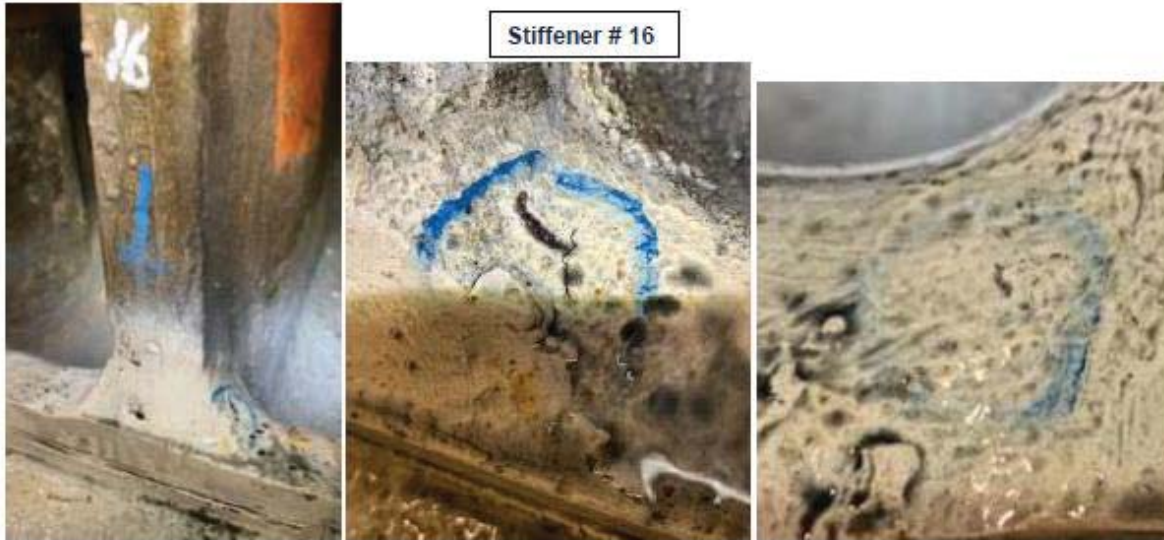
Figure 5-231: Head Cover, Small Stiffener Cracks
