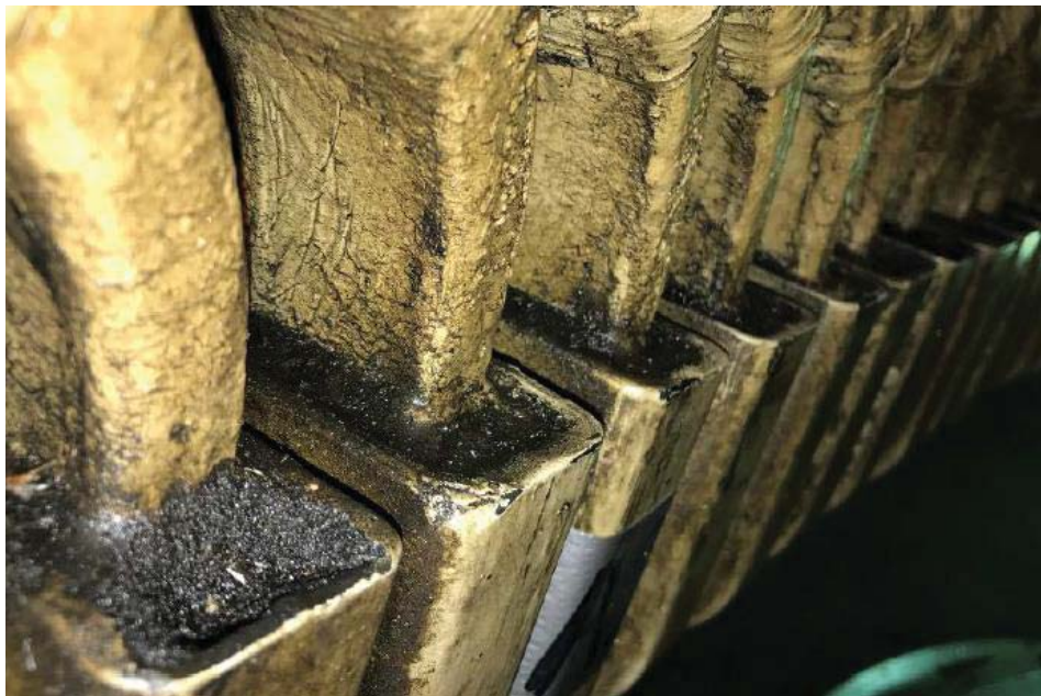
Figure 5-146: Stator Windings: Damaged End-Cap
