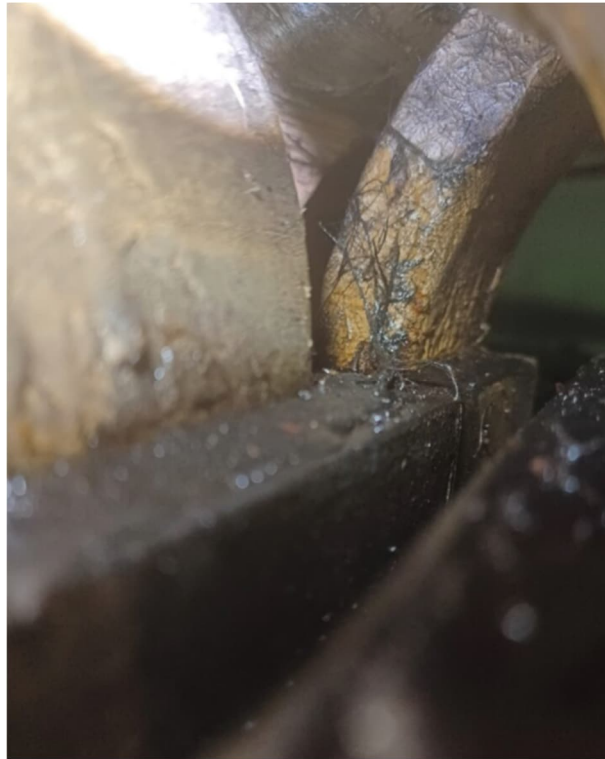
Figure 3-3: Fiberglass Sticking from Edge of Slot
