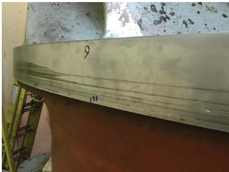
Figure 5-33: Runner Lower Wearing Ring, Contact Damage
