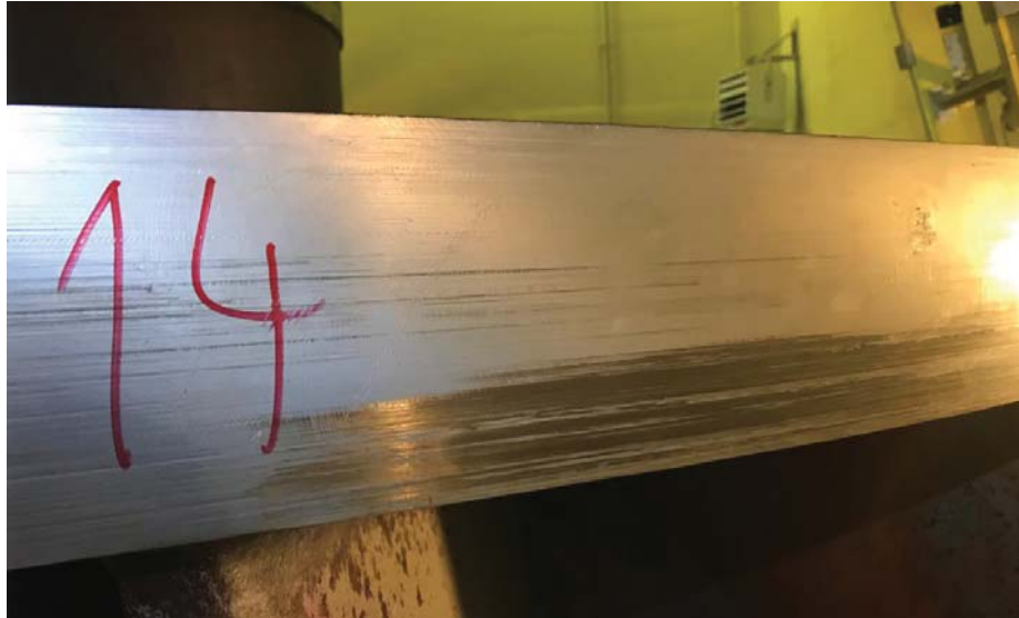
Figure 5-31: Runner Upper Wearing Ring, Contact Damage
